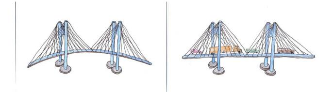
Weight Applied to a Suspension Bridge Will Flatten Out the Roadway
